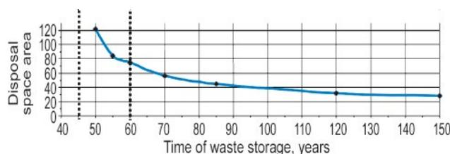
Figure 3. HWL disposal space area vs. HLW cooling time in a long-term storage facility (French HLW disposal project CIGEO, clay formations) [20]
