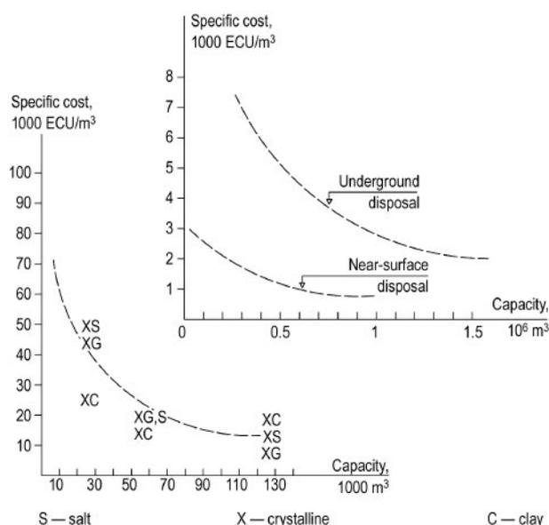
Figure 2. RW disposal cost vs. RW disposal facility's capacity (bottom left – for long-lived ILW and HLW, top right – for LLW and short-lived ILW) [16]
