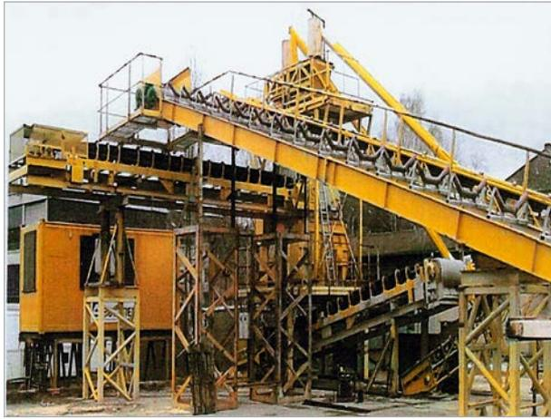
Fig. 3. Facility for 100% measurement of milled brick and stone with a capacity of 50 t/hour
