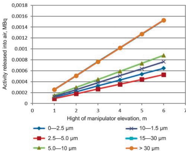
Figure 1. Dependence of the term source activity on the height of manipulator elevation for the considered diameter ranges
