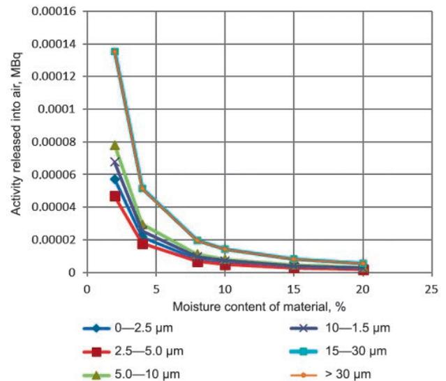
Figure 3. Dependence of the term source activity from the moisture content of material at a constant wind speed
