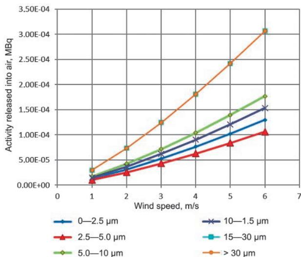
Figure 2. Dependence of the term source activity from the wind speed at a constant moisture content of material
