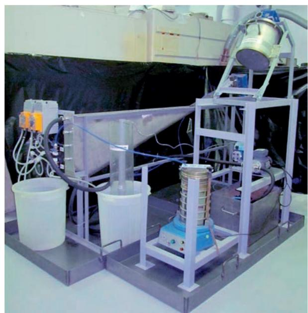
Figure 2. Laboratory test installation for RCS treatment via hydro-separation method
