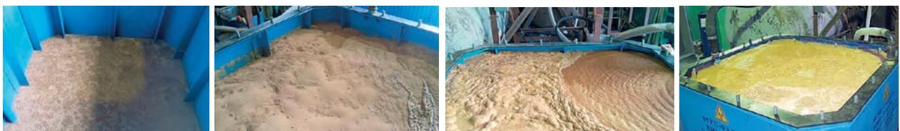
*Fig. 3. Container filling with sludge and IER dewatering*
